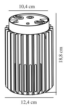
Voltage (V): 220-240 Volt IP degree: IP54 Maximum bulb wattage (W): 15 Class (Class 1, Class 2, Class 3): Class 1 (Earth contact) Socket type: E27
