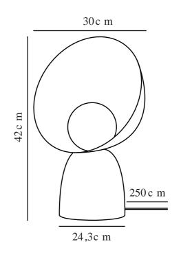
Voltage (V): 220-240 Volt IP degree: IP20 Maximum bulb wattage (W): 25 Class (Class 1, Class 2, Class 3): Class 2 (Double isolated) Socket type: E14 Switch placement: On the cable
