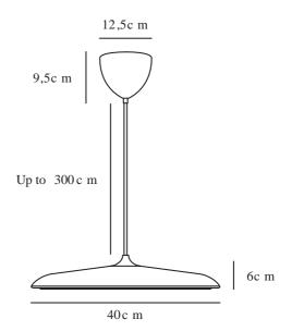
Voltage (V): 220-240 Volt IP degree: IP20 Class (Class 1, Class 2, Class 3): Class 2 (Double isolated) Socket type: LED – Nonreplaceable light source Parallel connection: False
