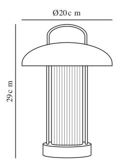
Voltage (V): 3,7 Volt IP degree: IP20 Class (Class 1, Class 2, Class 3): Class 3 (12V) Socket type: LED Module Switch placement: In the base Parallel connection: False
