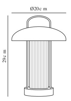
Voltage (V): 3,7 Volt IP degree: IP20 Class (Class 1, Class 2, Class 3): Class 3 (12V) Socket type: LED Module
