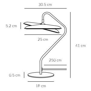
Voltage (V): 220-240 Volt IP degree: IP20 Class (Class 1, Class 2, Class 3): Class 2 (Double isolated) Socket type: LED – Nonreplaceable light source Switch placement: On the cable Parallel connection: False
