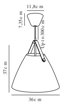
Voltage (V): 220-240 Volt IP degree: IP20
